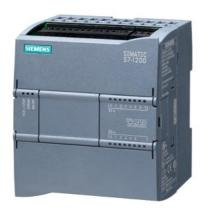
SIPLUS S7-1200 CPU 1212C DC/DC/DC based on 6ES7212-1AE40-0XB0 with conformal coating, -40...+70 °C, start up -25 °C, signal board: 0, compact CPU, DC/DC/DC, onboard I/O: 8 DI 24 V DC; 6 DQ 24 V DC; 2 AI 0-10 V DC, power supply: 20.4-28.8 V DC, program/data memory 75 KB
