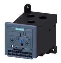
Overload relay 12.5...50 A Electronic For motor protection Size S2, Class 5E...30E Stand-alone installation Main circuit: Straight-through transformer Auxiliary circuit: Spring-type terminal Manual-Automatic-Reset Internal ground fault detection
