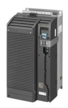
SIPLUS G120 PM240-2 IP20-FSE-A-400V 45 kW based on 6SL3210-1PE28-8AL0 with conformal coating, -20...+50 °C, with integrated class A filter with integrated braking chopper 380-480 V 3 AC +10/-20% 47-63 Hz power high overload: 37 kW at 200% 3 s,150% 57 s,100% 240 s power low overload: 45 kW at 150% 3 s,110% 57 s,100% 240 s 551x 275x 237 (HxWxD), FSE design, degree of protection IP20 without CU and operating unit released as of CU FW version V4.7 HF8
