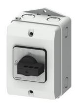
SENTRON switch disconnector 3LD in molded-plastic enclosure, repair and maintenance switch with EMC plate, 3-pole lu: 32A, AC23A 400V at 50/60Hz: 11,5kW, used with frequency converter: AC20 400V at 0-550Hz: 7,5kW, 1NO + 1NC 20-150ms leading, molded-plastic encapsulation for metric cable gland, knoboperated mechanism, black, lockable in 0- and I-position, incl. cable shield clamps
