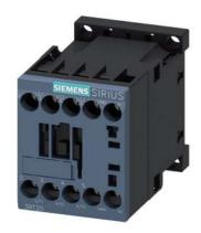
power contactor, AC-3e/AC-3, 9 A, 4 kW / 400 V, 3-pole, 230 V AC, 50/60 Hz, auxiliary contacts: 1 NO, screw terminal, size: S00, upright mounting position
