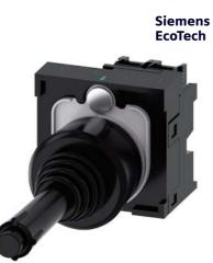
Coordinate switch, 22 mm, round, plastic, black, 2 switch positions, vertical, momentary contact type, with mechanical interlocking in O position, with holder, 1 NO, 1 NO, screw terminal
