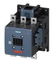
power contactor, AC-3e/AC-3 300 A, 160 kW / 400 V, AC (50-60 Hz) / DC Uc: 220-240 V 3-pole, auxiliary contacts 2 NO + 2 NC permanently mounted drive: conventional main circuit: busbar control and auxiliary circuit: screw terminal
