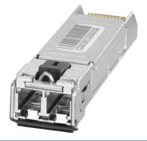
SCALANCE X accessory; plug-in transceiver SFP991-1LD; 1x 100 Mbit/s LC port, optical; single-mode optical up to max. 26 km 1 pack = 10 units.
