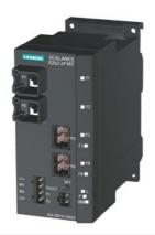
SCALANCE X202-2P IRT managed IE IRT switch, 2x 10/100 Mbps RJ45 ports, 2x 100 Mbps POF SC RJ ports, error signaling contact with set pushbutton, redundant power supply, PROFINET IO device, network management, Redundancy Manager integrated, incl. electron. manual on CD-ROM, C-PLUG optional
