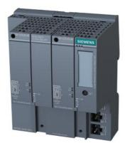
XF202-2P IRT managed IE IRT switch, 2x 10/100 Mbit/s RJ45 ports, 2x 100 Mbit/s POF SC RJ Ports, Bus adapter assembled, Error signaling contact with set pushbutton, redundant power supply, PROFINET IO device, network management, Redundancy Manager integrated, incl. electron. manual on CD-ROM, C-PLUG optional.
