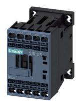
traction contactor, AC-3e/AC-3, 12 A, 5.5 kW / 400 V, 3-pole, 24-34 V DC, 0.7-1.25\* Us, electronic drive, with integrated varistor, auxiliary contacts: 1 NC, spring-loaded terminal, size: S00
