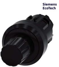
stop button, 22 mm, round, plastic, black, pushbutton raised, latchable after pushing in by rotating clockwise, unlatches when turned counterclockwise
