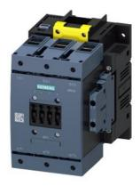
power contactor, AC-3e/AC-3 115 A, 55 kW / 400 V, AC (50-60 Hz) / DC Uc: 96-127 V x (0.8-1.1) F-PLC input 24 V DC 3-pole, auxiliary contacts 2 NO + 2 NC drive: electronic main circuit: box terminal control and auxiliary circuit: screw terminal
