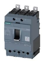
circuit breaker 3VA4 UL frame 125 breaking capacity class S 25kA @ 480 V 3-pole, line protection TM210, FTFM, In=110A overload protection Ir=110A fixed short-circuit protection Ii=10 x In clamp connection
