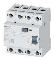
Residual current operated circuit breaker, 4-pole, type A, In: 125 A, 30 mA, Un AC: 400  $\rm V$
