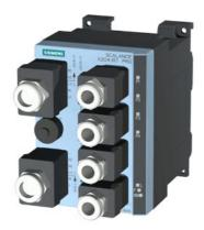
SCALANCE X204IRT PRO, managed IE IRT switch with degree of protection IP65/67, 4x 10/100 Mbps push-pull RJ45 ports, error signaling contact with set push-button; redundant power supply; PROFINET IO device, network management, Redundancy Manager integrated, incl. electron. manual on CD-ROM, C-PLUG optional
