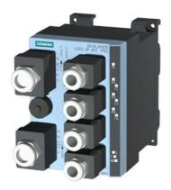
SCALANCE X201-3P IRT PRO; Managed IE IRT switch Degree of protection IP65/67; 1x 10/100 Mbps push pull RJ45 port; 3x 100 Mbps push-pull SCRJ port; Error signaling contact with set pushbutton; Redundant power Supply; PROFINET IO device; network management; Redundancy Manager integrated, incl. electron. manual on CD-ROM, C-PLUG optional
