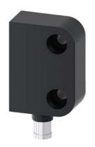
magnetically-operated switch contact block, rectangular small 26 x 36 mm, for door hinge left, contacts: safety contacts 1 NO+1 NC signaling contact 1 NC (31-32), with 8 mm latching connection connector 6-pole, without LED the matching solenoid 3SE6714-3CA or offset by  $90^\circ$  3SE6724-3CA
