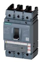
circuit breaker 3VA5 UL frame 250 breaking capacity class H 65kA @ 480V 3-pole, line protection TM230, FTAM, In=225A overload protection Ir=225A fixed short-circuit protection Ii=5...10 x In without connection
