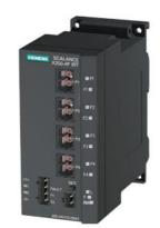
SCALANCE X200-4P IRT managed IE IRT switch, 4x 100 Mbps POF SC RJ ports, error signaling contact with set pushbutton, redundant power supply, PROFINET IO device, network management, Redundancy Manager integrated, incl. electron. manual on CD-ROM, C-PLUG optional
