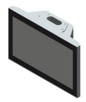
SIMATIC HMI TP1500 Comfort Pro, support arm, neutral front, Comfort Panel, Touch operation, 15" widescreen TFT display, 16 million colors, PROFINET interface, MPI/PROFIBUS DP interface, 24 MB configuration memory, WEC 2013, configurable from WinCC Comfort V14 SP1 with HSP
