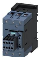
power contactor, AC-3e/AC-3, 80 A, 37 kW / 400 V, 3-pole, 110 V AC, 50/60 Hz, auxiliary contacts: 2 NO + 2 NC, screw terminal, removable auxiliary switch
