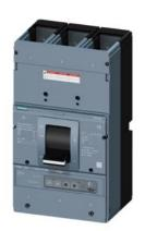
circuit breaker 3VA6 UL frame 1200 breaking capacity class H 65kA @ 480 V 3-pole, line protection ETU350, LSI, In=1200A overload protection Ir=500A - 1200A short circuit protection Isd=1,5-10 x Ir, Ii=1,5 x In w/o connection
