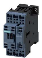
Contactor, AC-3, 18.5 kW / 400 V, 1 NO + 1 NC, 24 V DC with varistor 3-pole, Size S0 Spring-type terminal
