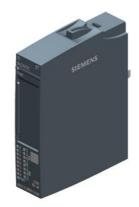
SIPLUS ET 200SP DI 8x24 V DC SRC BA based on 6ES7131-6BF61-0AA0 with conformal coating, -40...+70 °C, digital input module, suitable for BU type A0, color code CC02, source input, (NPN, sourcing input) input type 1 (IEC 61131), input delay 0.05..20 ms module diagnostics for: supply voltage
