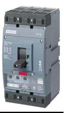
CIRCUIT BREAKER 3VT2 HIGH BREAKING CAPACITY ICU=36KA, 415V AC 3-POLE; CIRCUIT BREAKER W/OVERCURRENT RELEASE SYSTEM PROTECTION ETU DP, LI IR= 40...100A, OVERLOAD PROTECTION IRM= 4... 8KA SHORT-CIRCUIT PROTECTION, WITHOUT AUXILIARY RELEASE WITHOUT AUXILIARY/ALARM SWITCH
