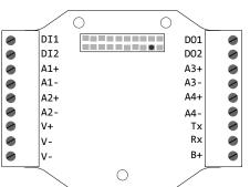
B+. 3.6 V DC to 5.5 V DC (use for battery powered models only) RX/-. Serial communication line for the Gateway. No connection for Nodes
