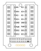
Ax+ and Ax-. Analog IN x. Analog inputs for devices requiring more than one connection, such as thermocouples or RTDs. When there is no Ax-, use Ax+ as an analog input. DIx. Discrete IN x
