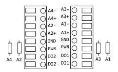
Ax+ and Ax-. Analog IN x. Analog inputs for devices requiring more than one connection, such as thermocouples or RTDs. When there is no Ax-, use Ax+ as an analog input.
