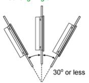
When installing the panel in a slanted position with an incline more than 30 $^{\circ}$ , the ambient temperature must not exceed 40 $^{\circ}$ C (104 $^{\circ}$ F). You may need to use forced air cooling (fan,A/C) to ensure the ambient operating temperature is 40 $^{\circ}$ C or less (104 $^{\circ}$ F or less).
