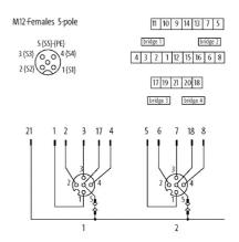
free arrangeable, contact 1:1 on terminals for 5 signals per port, possibilty to bridge each PIN5  $\,$
