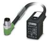
Sensor/actuator cable, 3-position, PUR halogen-free, black-gray RAL 7021, Plug angled M12 SPEEDCON, coding: A, on Valve connector BI (11 mm), with 1 LED, connected with Z diode, cable length: 0.3 m
