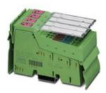
Inline, Digital output terminal, Digital outputs: 8, 24 V DC, 2 A, connection technology: 4-conductor, transmission speed in the local bus: 500 kbps, degree of protection: IP20, including Inline connectors and marking fields
