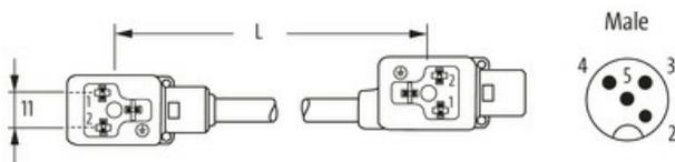
Valve plug 2      Valve plug 1      Male M12
