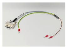
Y-ADAPTER CABLE FOR DEVICES WITH RS485 INTERFACE AND SUB-D CONNECTOR ON 2 X RJ45- FEMALE CONNECTOR FOR MOUNTING ONES RS485-BUS WITH PATCH CABLE 2-CORE, TWISTED, SHIELDED, LENGTH: 0.3M 1 X SUB-D PIN 9-POLE ON 2 X RJ45 SOCKET 8-POLE
