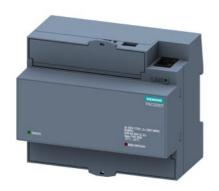
SENTRON, measuring device, 7KM PAC3200T, strd mnt. rail encl. w/o display, L-L: 400 V, L-N: 230 V, 5 A, strd rail instr., 3-phase, MODBUS TCP, apparent /active/reactive energy, wide-range pwr sup. unit AC/DC, screw terminals
