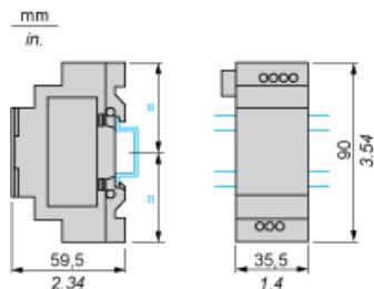
Screw Fixing (Retractable Lugs)
